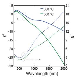
Fig. 2. Dielectric functions of titanium nitride films deposited at 300  $^{o}C$  and 500  $^{o}C$  retrieved by spectroscopic ellipsometry measurements. The films were deposited with the flow ratio of argon and nitrogen set to 4:6.
