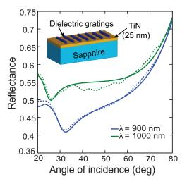
Fig. 11. Angular reflectance of dielectric (ZEP, electron-beam resist) gratings formed on top of a 30 nm thick film of TiN. The inset shows the geometry of the structure. The measured (solid lines) and calculated (dashed lines) reflectances are plotted against angle of incidence for two different wavelengths.
