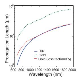
Fig. 7. Propagation length of the lowest order symmetric SPP mode in a metal/air/metal waveguide with an air gap of 300 nm for different metals: TiN, gold (JC) and gold with loss factor of 3.5.
