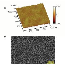
Fig. 5. Characterization of 30 nm thick TiN film deposited on a c-sapphire substrate. a) Atomic force microscope (AFM) image b) Scanning electron micrograph.
