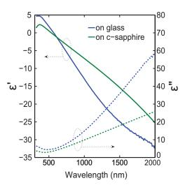
Fig. 3. Dielectric functions of titanium nitride films deposited at 300  $^oC$  on glass and c-sapphire substrates.
