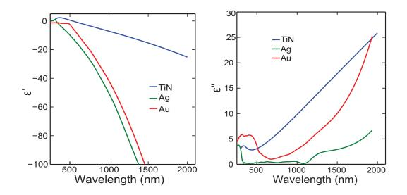
Fig. 10. Dielectric function of TiN in comparison with conventional plasmonic materials: gold and silver (data adapted from JC [21, 39]).
